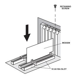
Figure 3: Installing The Modem
